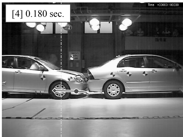
Fig.2 Sequence of Collision and Parts' Drop in Rear-end Collision Test (No.3, 35km/h)
