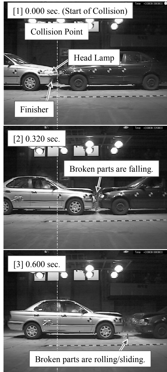
Fig.5 Sequence of Collision and Parts' Drop in Frontal Collision Test
