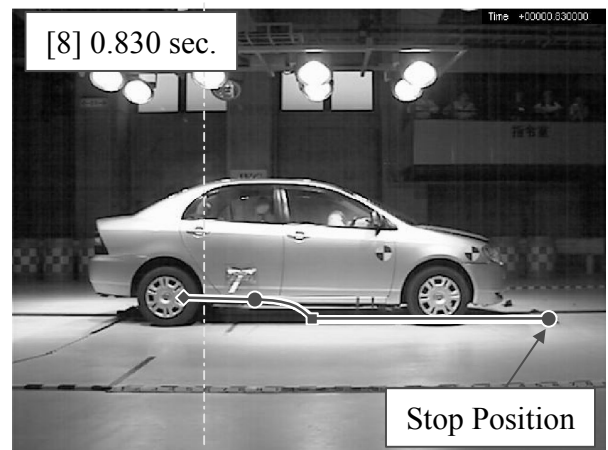
Fig.2 Sequence of Collision and Parts' Drop in Rear-end Collision Test (No.3, 35km/h)
