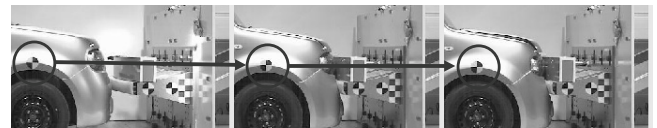
Fig. 6 Trace the Target on the Front Fender by Motion picture Analyzer
